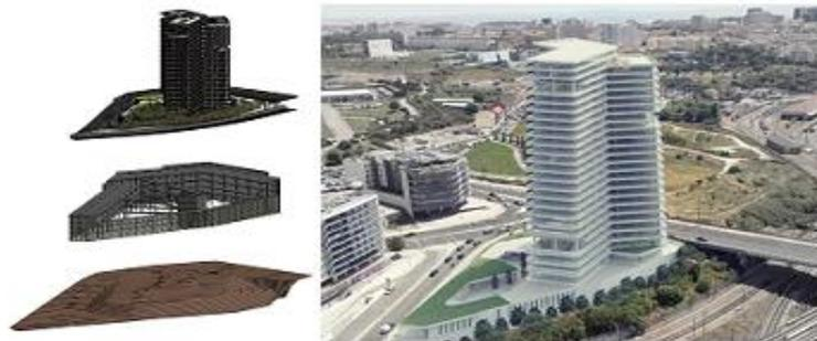
**Fig. 2.** – 3D Architecture BIM model and the Retaining BIM model (left) and virtual view of the future tower (right)
