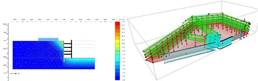
**Fig. 3.** Analysis in PLAXIS2D (left) and SAP2000 model, the last imported from a BIM file
